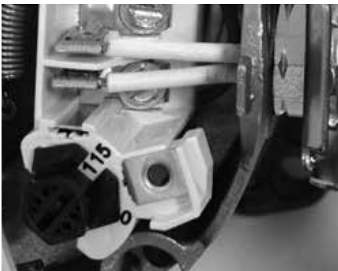
Figure 4: Motor Set for 115 Volt Operation
